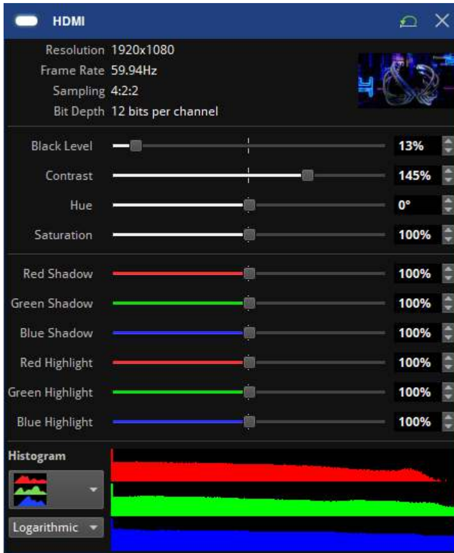
Figure 9-7. Adjusting the contrast control will make brighter areas appear closer to the 100% threshold, assuming some areas contain white content in the image and is desirable
