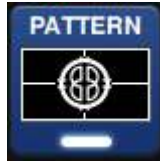
Figure 11-3. Test Pattern pipeline tile, indicating the current active test pattern
