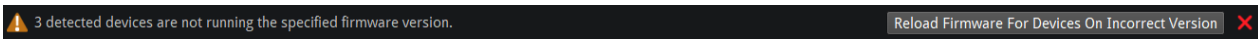
Figure 15-11. Error message notification shown when detected fixtures are running incorrect firmware versions
