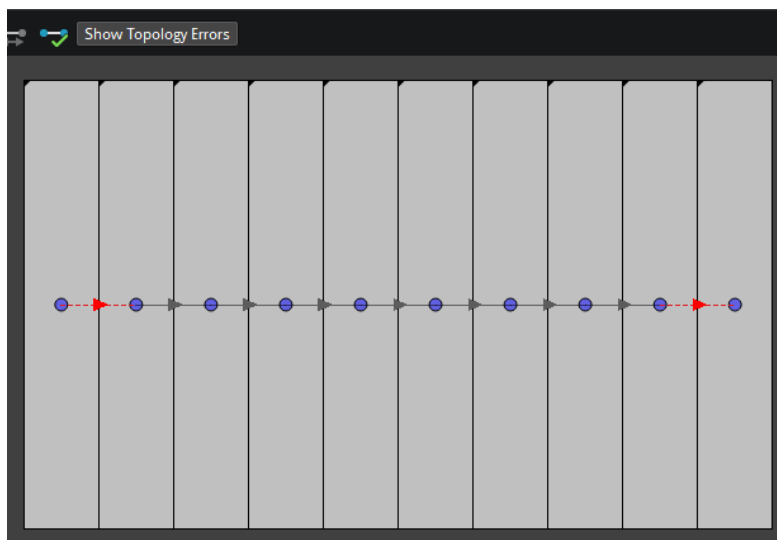
Figure 7-28. Example of incorrect topology, notice the arrows on the far left and right are highlighted in red
