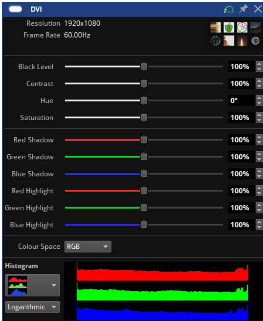
Figure 9-5. A fairly washed out incoming signal on DVI (see thumbnail top left) with the corresponding histogram for red, green and blue when the Input
