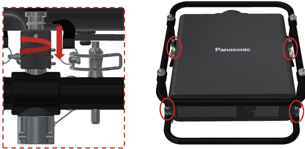
Figure 14 Tighten the four attachment nuts
