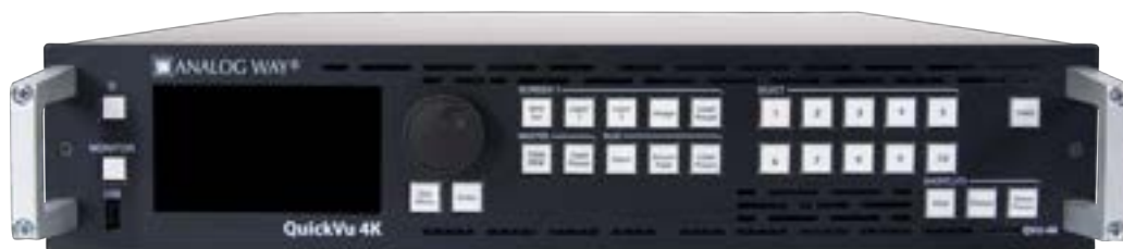
Fig. 2 - QuickVu 4K front panel
