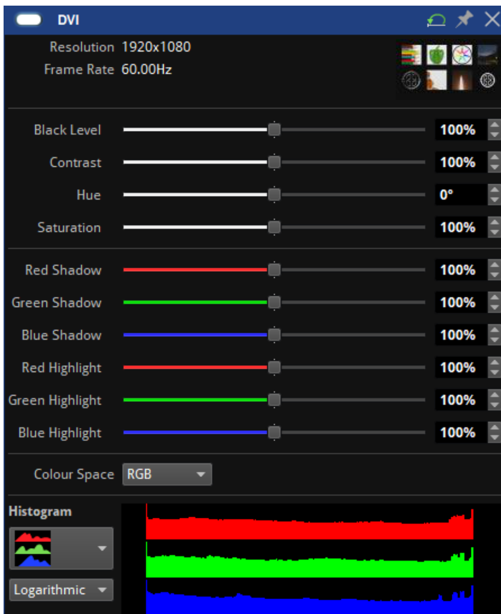
Figure 9.12 - A fairly washed out incoming signal on DVI (see thumbnail top left) with the corresponding histogram for red, green and blue when the Input
