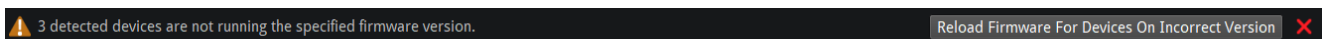
Figure 14.14 - Error message notification shown when detected fixtures are running incorrect firmware versions
