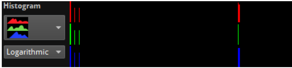
Figure 9.11 - Test pattern showing colour bars at 75% and the corresponding Logarithmic RGB histogram
