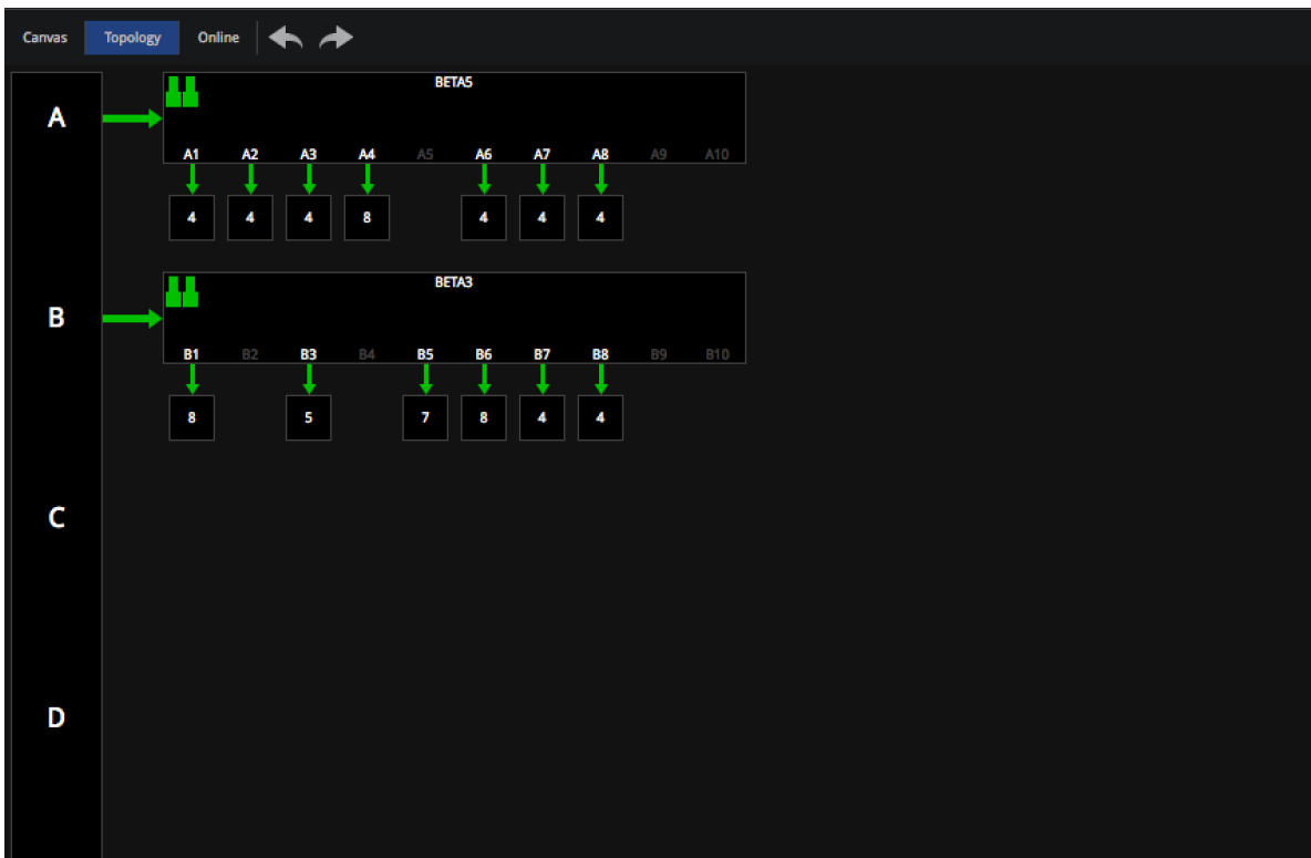
Figure 8.18 - Topology View with Fixtures connected to XD Units connected to SX40 ports A and B
