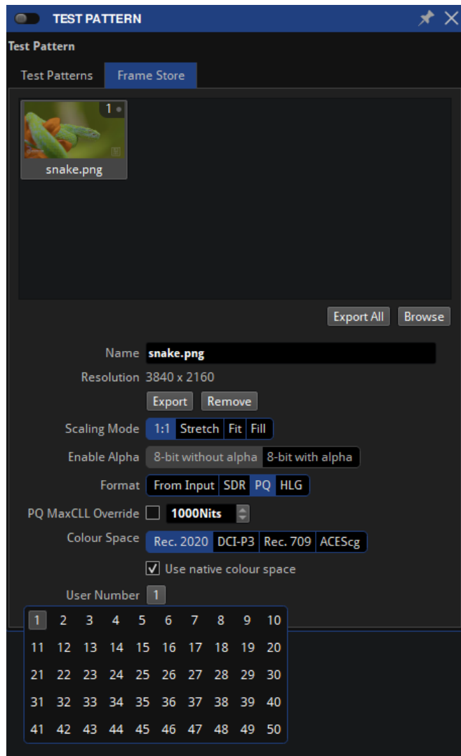
Figure 11.10 - Frame Store properties with user number range and PQ Max CLL Override.
